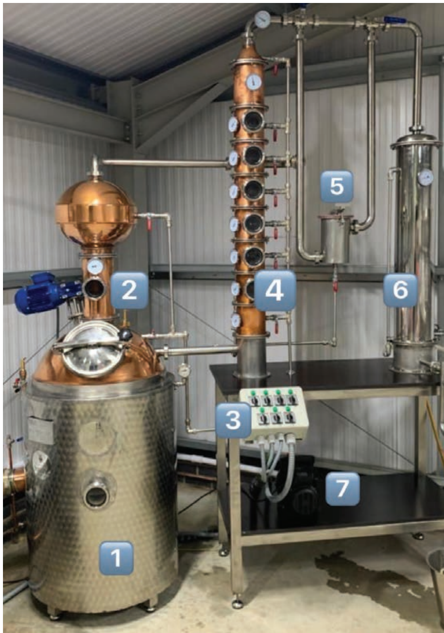
GIN DISTILLING PROCESS IN NUMBERS: 1) WATER JACKET HEATED BY TWO ELEMENTS USING SIX HEATERS. 2) COPPER POT STILL OF 120L CAPACITY CALLED ANGELICA WITH MIXING PADDLE. 3) CONTROL PANEL. 4) SIX PLATE RECTIFICATION COLUMN, USED TO STRIP THE FLAVOUR OF WASTE ALCOHOL AND TURN IT BACK INTO A USEABLE BASE SPIRIT. 5) VAPOUR INFUSION BASKET: "WHEN DISTILLING BURRELL'S DRY GIN WE ADD KEY BOTANICALS AT THIS POINT TO GIVE FURTHER DEPTH TO THE SPIRIT DURING DISTILLATION." 6) CONDENSER: MANY TUBES FILLED WITH RUNNING COLD WATER, VAPOUR PASSES THROUGH AND CONDENSES THIS BACK INTO LIQUID WHICH IS COLLECTED VIA THE PARROT DISH. 7) CIP (CLEAN IN PLACE) PUMP, USED TO CLEAN THE EQUIPMENT AFTER EACH USE
